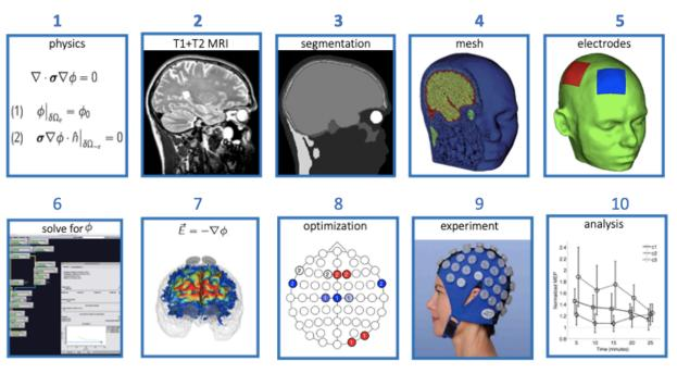
Schematic of the steps involved in electromagnetic brain stimulation research, including the physics equations to solve (1), the process of building a finite element head model from MRI scans (2-5), calculation of the electric potential and field (6-7), computational optimization of currents to achieve a desired field (8), and testing the results in experiments with human volunteers (9-10).
